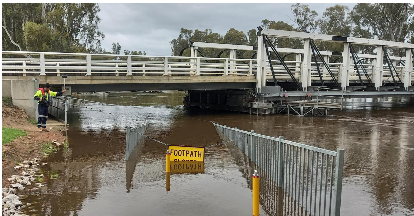
A LMW staff member checks river flood heights to compare against LMW infrastructure heights.
